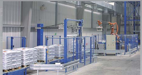
e.g. turnkey bag-filling line with over 1,000 bags filled and palletised per hour
