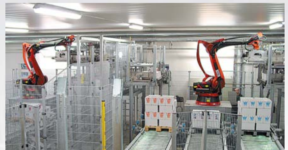
e.g. fully automatic palletising centre for milk trays with the 2 redundant master computers connected to the customer's superordinate SAP-R/3 system
